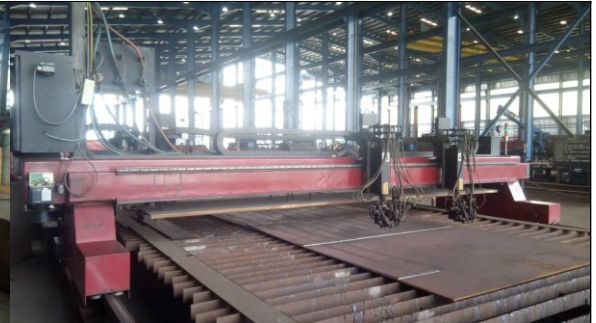
CNC Machine for Plates Cutting
