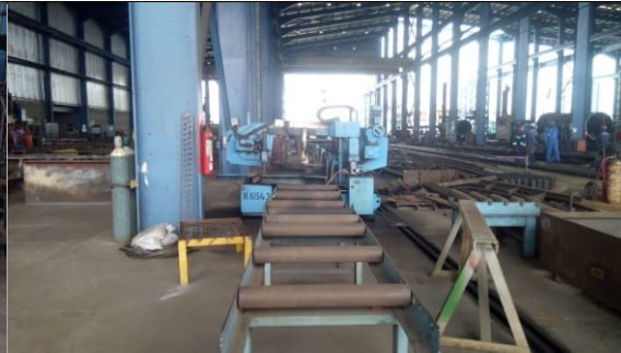
Cool Cut Machine for Cutting Pipe
