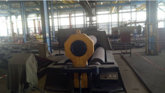
Rolling Machine for Folding Plate to Pipe Shape or Vessel
